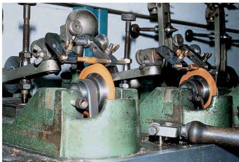
Figure 9. In this photo of a mechanical sawing operation, two machines are shown. The sawing machine controls the lowering of the crystal, attached to a dop, onto a thin copper blade that is revolving at a high speed. Photo by James E. Shigley.
